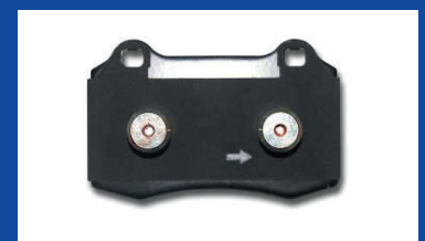
The arrows should follow the direction of disc rotation.
