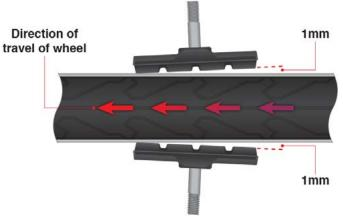
The half moon can be accompanied by a directional arrow, however if this is not present the cut out will appear on the leading edge of the pad. It is imperative that this crescent/cut-out runs horizontally across the brake disc, and should be located on the leading edge to ensure even pad wear and the correct distribution of force across the brake pad surface. This reduces pad oscillation and thus prevents noise.
