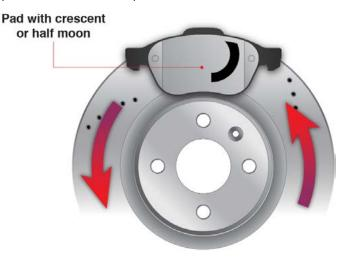
If this type of pad is fitted in the opposing direction then you are highly likely to experience noise as the leading edge will contact the disc first, causing chatter, heard by the fitter or customer as a high pitch squeal.
