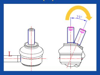
The LH stabiliser will be marked with an "L".
