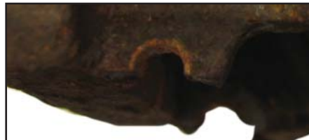
Damaged / Cut Pin Holes: examples LCA / RCA 348, 365, UCA 230
