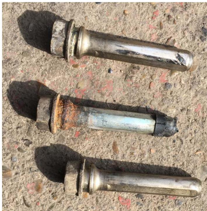
*\*Anything interrupting free movement of brake components will interrupt the even material transfer process, leading to excessive DTV eventually resulting in brake judder.*
