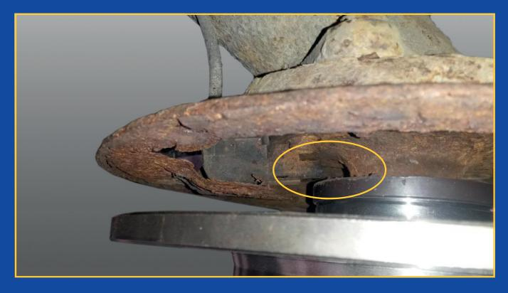
To fix this issue, remove the ABS sensor from its mounting point and remove the corrosion before refitting the sensor and the new disc.
